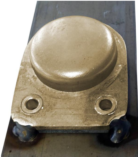
Correctly welded “spot” welds
