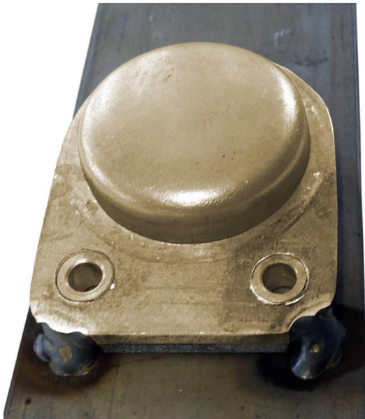
Correctly welded "spot" welds
