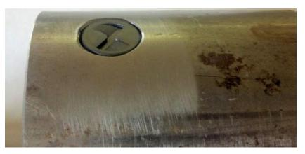
Close-up of an **STI** tag mounted into a pipe; notice that the tag is mounted flush to the surface of the pipe. Recessing the tag into the pipe deeper than shown may adversely affect the ability to interrogate the tag.
