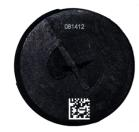
Information has been laser-etched onto the tag.
