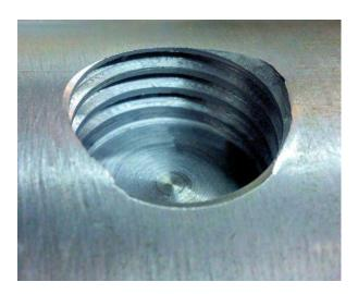
A mounting hole has been end-milled and bottom-tapped into the sidewall of a pipe.
