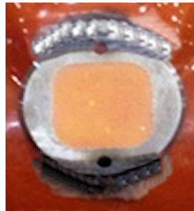
Incorrectly welded - too far around tag
