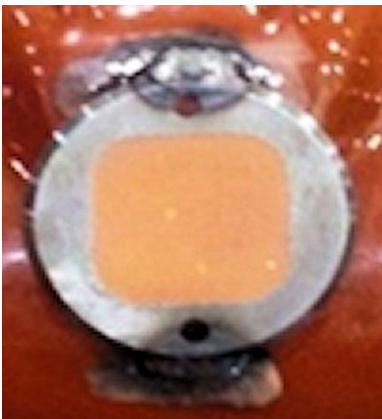
Correctly welded "spot" welds
